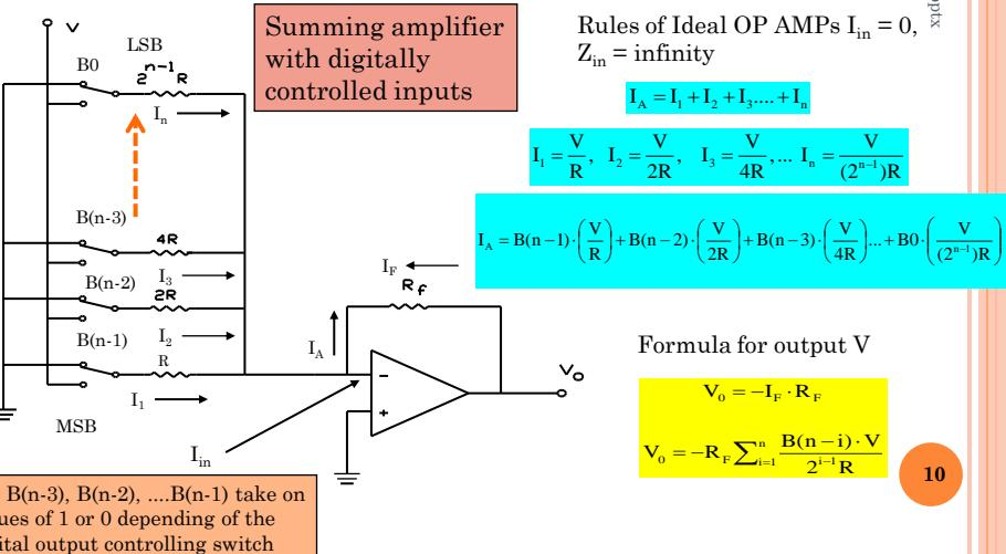
B0, B(n-3), B(n-2), ..., B(n-1) take on values of 1 or 0 depending on the digital output controlling switch
