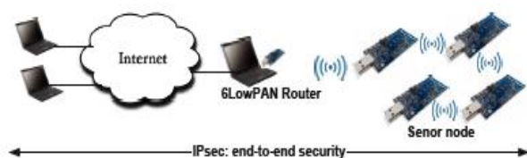
Fig. 1: Use of IPsec to secure communication between sensor nodes and hosts in an IPv6 enabled internet. [4]
