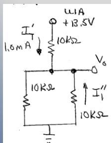
$$I''_1 = -1.0\text{mA} \left[ \frac{10\text{k}\Omega}{10\text{k}\Omega + 10\text{k}\Omega} \right] = (-1.0\text{mA})(0.5)$$
